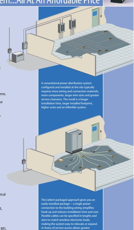
location flexibility and smaller installed footprint. And since the power source is right there in the room, it eliminates difficulties in establishing a proper ground. The system also eliminates potentially harmful harmonic neutral current from the building wiring system.
